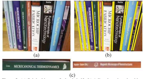
Figure 3: (a) Original image of a bookshelf. (b) A line detection algorithm is used to find the spine boundaries from the original image. (c) The extracted book spines are reprojected into rectangle regions.
