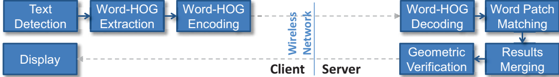
Figure 5: Overview of the querying process of the image-based retrieval system that uses visual text information.
