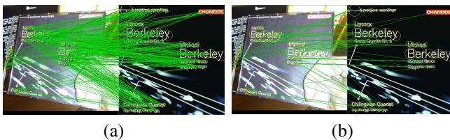
Figure 4. (a) Pairwise feature matches using the recognized character. (b) Pairwise feature matches using word distances.
