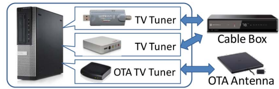
Fig. 2: A recording station consists of a PC and TV tuners that capture video from cable boxes and over-the-air antennae.
